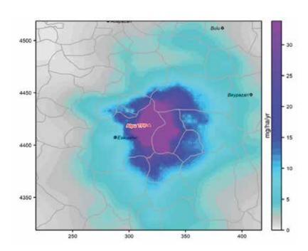
Figure 22. Estimated annual mercury accumulation (mg/m³) from Alpu CPP
